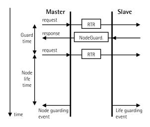
Guard time: time between 2 RTR. Node life time: max device response time.
